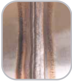
MIG-Double Pass As-welded
