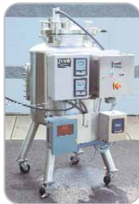
100 liter ASME Mammalian (CHO) Cell Culture Vessel. Magnetic mixer, differential level control, pH and conductivity controls, dissolved O 2 /O 3 instrumentation.
