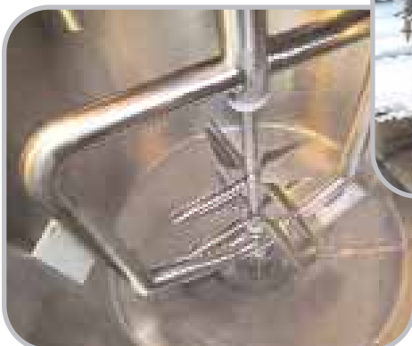
Interior view, Dual Motion Scrape Agitator with Sanifoil Impellers.
