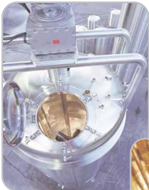
ASME Aerobic Fermentation Vessel 100 HP microbial agitator.
