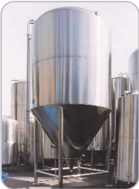
50 BBL Fermenter with bottom cone manway.
