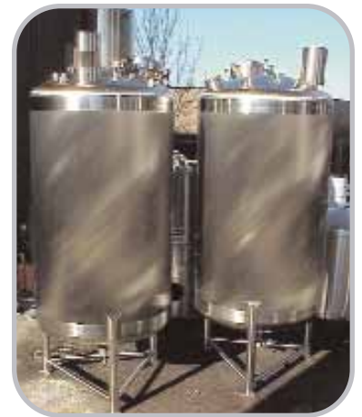
Batch Process Tanks with stainless steel mixers.
