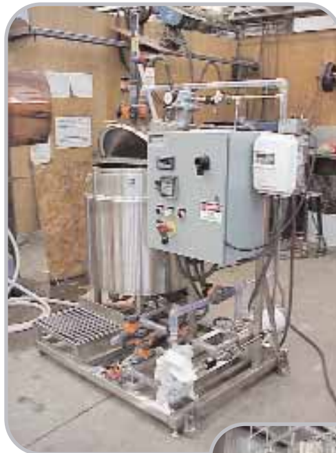
Sanitary Color Supply Blending Skid.
