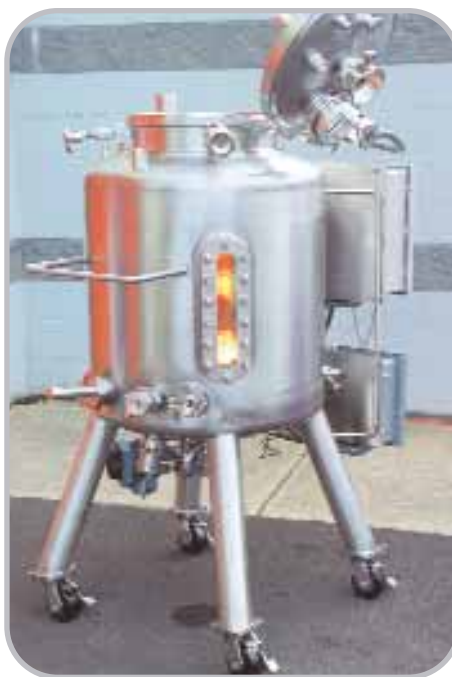
100 liter ASME Mammalian (CHO) Cell Culture Vessel. Magnetic mixer, differential level control, pH and conductivity controls, dissolved O 2 /O 3 instrumentation.
