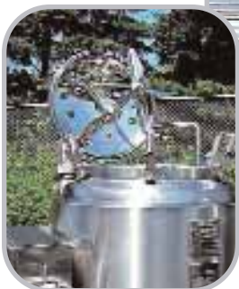
Pilot Reactor with lid-mount mixer.
