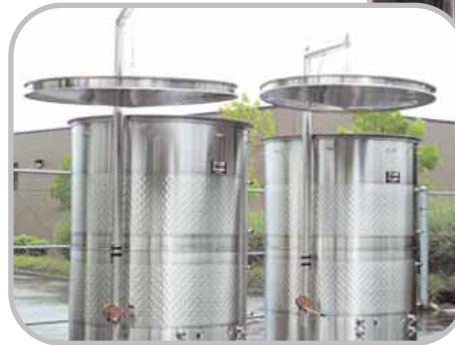
Variable Capacity Wine Tanks.
