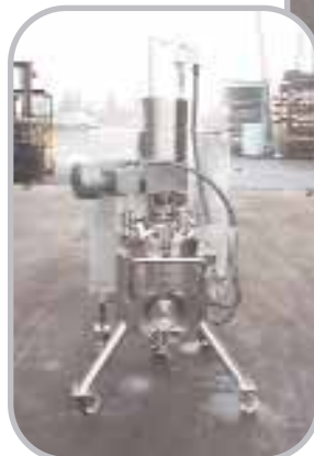
Ointment Processor, full scrape mix tank batch homogenizer.
