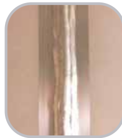
MIG-Double Pass Buffed/Polished 2B Mill finish
