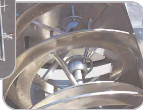
Interior view, Double Helix Ribbon Blender, counter rotating scrape.
