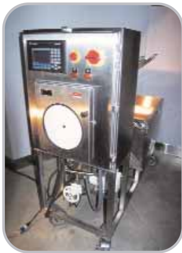
Water Recirculation Bath, PLC based technology.
