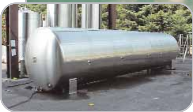
Water for Injection (WFI) 25,000 liter Storage Vessel. ASME, SIP/CIP, electropolished interior, expansion mount saddle supports.
