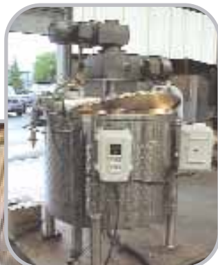
Cosmetic Mix Tank with tank-mounted agitator speed control.
