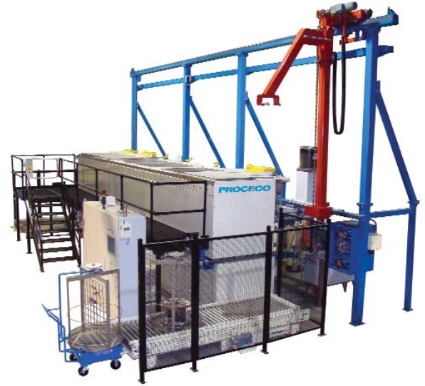
6-stage automated ultrasonic immersion degreasing line featuring automatic basket loading/unloading and convection drying.
